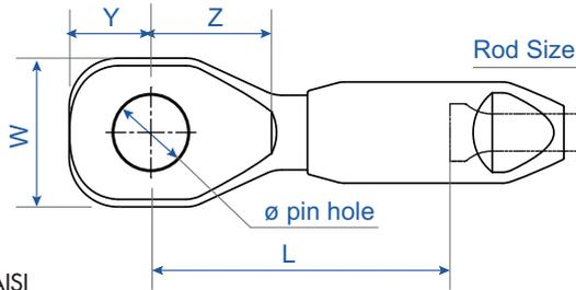
Material: Acidproof Stainless Steel / Matériau : Inox 316 AISI
