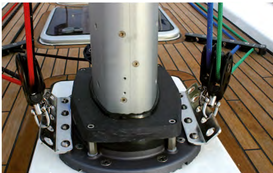
Deck collar including wedging and deck waterproofing, as well as the halyard blocks for keel stepped masts.
