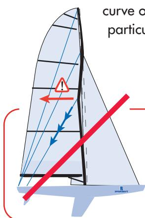
the babystays adjust the bend of the mid-section of the mast. If they are too tight in relation to the backstays, they can cause the inversion of the mast bend.
