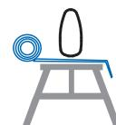
The **centre of gravity of the mast** (where it is balanced to work on) is defined by a red mark on the mast packing. Indicate this mark (after unpacking) with a strip of red tape.
