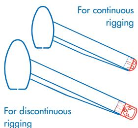
Attach the tip fittings to the ends of the spreaders (continuous and/or discontinuous), so they can receive the top and intermediate shrouds.
