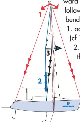
1. adjust the rake with the forestay, then tighten the backstay (cf 13.1);
