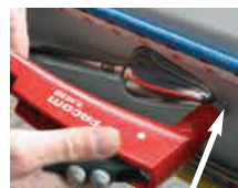
fixing a safety rivet
